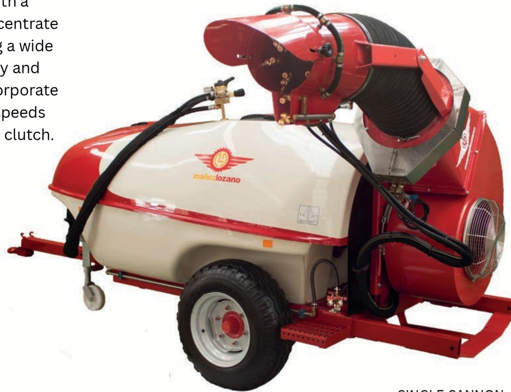
SINGLE CANNON It has a 90° vertical rotation and 360° horizontal rotation
